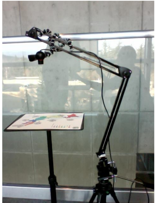
Figure 2: Shown above is a picture of the fiducial tracking interface. Above the computer monitor is a small consumer grade video camera, which is pointed downwards in order to view the fiducial markers which are placed on a printed paper map.
